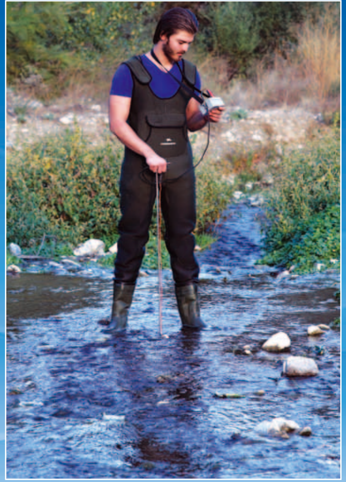
Measuring water velocity in the small river.
