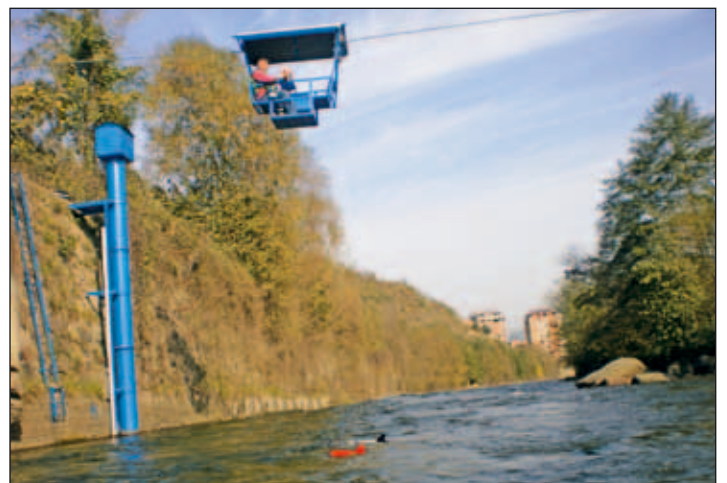
Pic.10: Current Meter CM-32 with 50 kg Single-drum winch (Teleferik).
