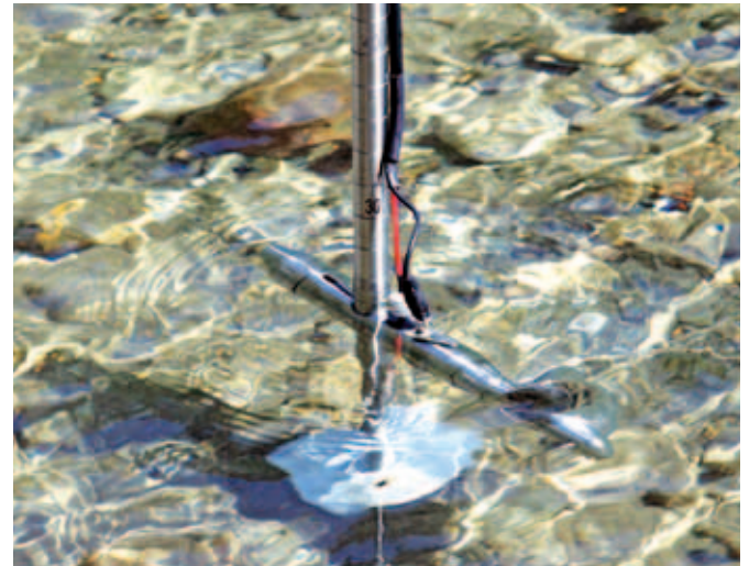
Pic.1: CM- 32 Current Water on rod 20 mm dia.
