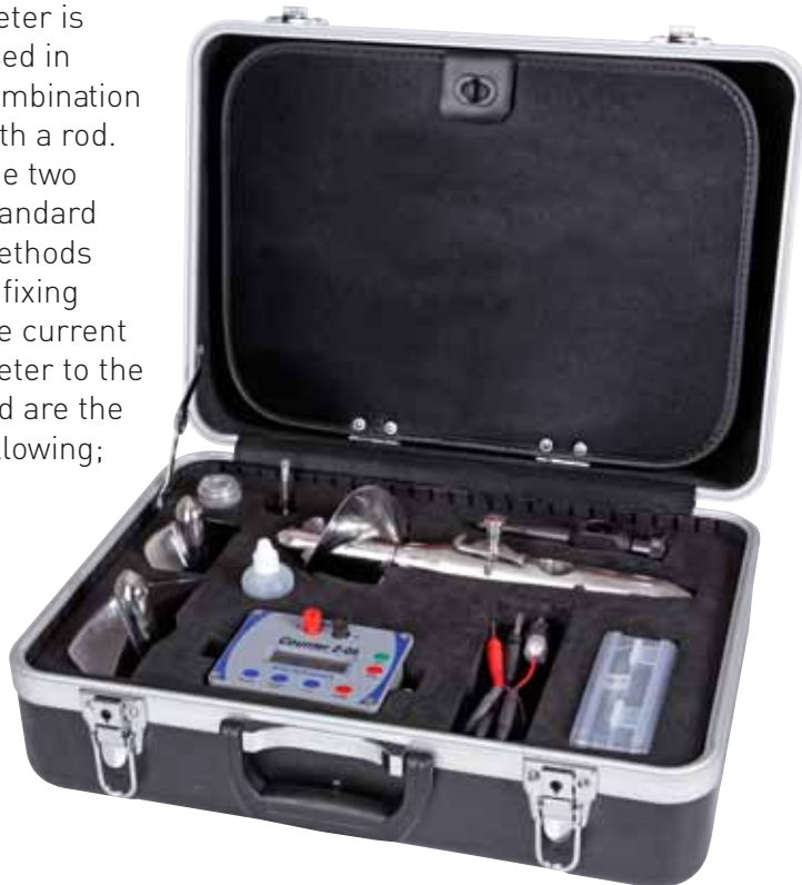
Pic.1: CM- 32 Current Water on rod 20 mm dia.
